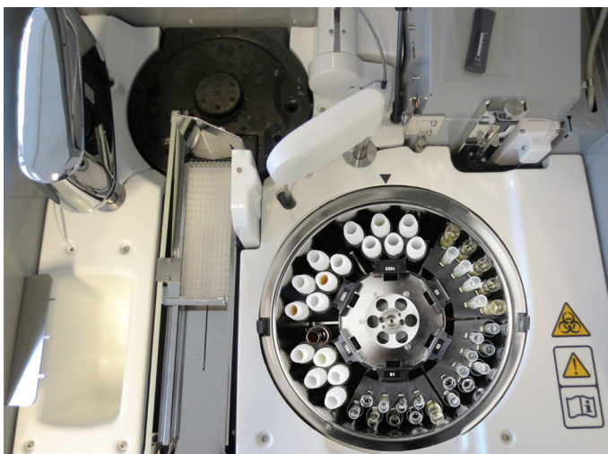
Indiko system includes combined sample and reagent disk for max 6 racks: 9- or 18-position sample racks and 6-position reagent racks.
